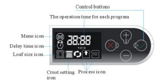
As soon as the bread maker is plugged into the outlet, a beep will be heard and "3:00" will constantly display with backlight, and the Menu icon will display and flash "01" which is the default program. The backlight will be extinguished if without any action within 15s.
